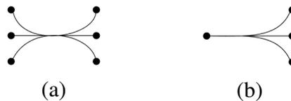
Figure 2: Type of bundles: (a) multiple source and destination nodes; (b) one common ending node.
